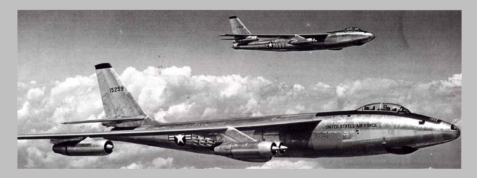
Relatively large numbers of the RB-47E were produced, this being a photo-reconnaissance version of the Stratojet bomber. Its primary purpose was to map the approaches to Soviet targets to aid planning nuclear bombing raids.
